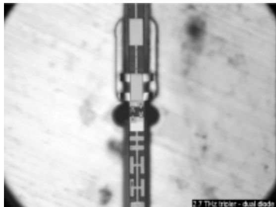
Fig. 3. Left: MOMED tripler shown mounted in waveguide block lower half. Output waveguide is above center, input backshort cavity below center. Right: Blow up showing output waveguide region with mounted antiparallel-pair membrane diodes.
