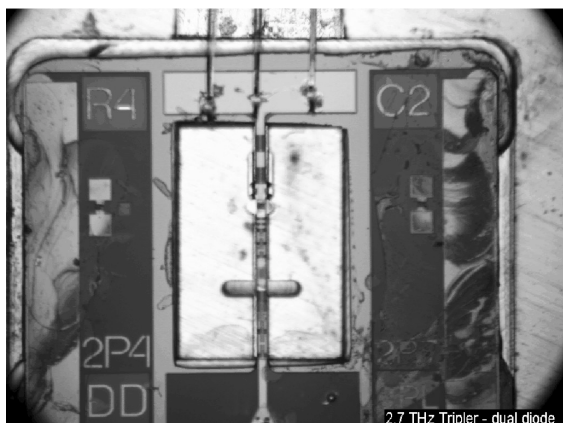
Fig. 3. Left: MOMED tripler shown mounted in waveguide block lower half. Output waveguide is above center, input backshort cavity below center. Right: Blow up showing output waveguide region with mounted antiparallel-pair membrane diodes.
